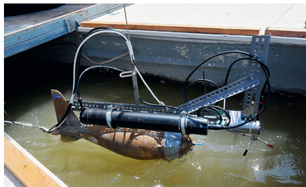
Figure 4. Comparison of different monitoring devices to determine suspended sediments during a joint measurement: US-P61-A1 suspended sediment sampler, Acoustic Doppler Velocimeter (ADV) and turbidity sensor
