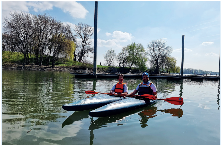
Figure 4. The recycled riverine litter can take surprising forms. Riversaver kayaks are made out of environmental plastics, mainly the polyethylene fraction of the plastic pollution collected on the river Tisza. Credit: Eniko Kubinyi
