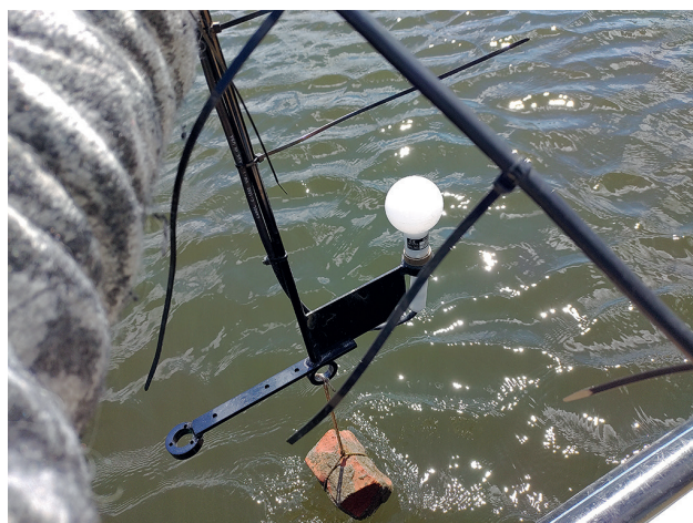
Figure 1. LI-COR underwater spherical PAR sensor (left; PAR plane air sensor not shown; Lacul Babina) and measurement of underwater light below filamentous algal mats and leaves of Nymphaea alba , respectively (right, Lacul Ligheanca).
